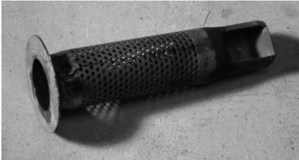
The last muffler with endplate from another angle. Unpainted. Paint with high temp black colour.
